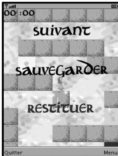
**Figure 10-8.** A custom menu using `lcdui` commands instead of softkeys
